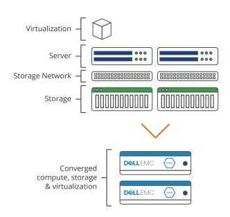
The VxRail platform converges Dell's PowerEdge servers and VMware's vSAN technology in simple, scalable building blocks that leverage VMware's full suite of management tools.
